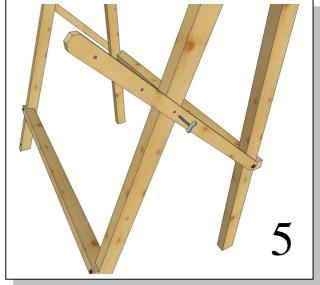
5. The wing screw is fastened in one of the 3 holes and the side batten is turned down and fastened to the back leg. The 3 holes gives the target stand different angles. The innermost hole (appr. 3° angle) is great for short distance shooting, the middle hole (appr. 8° angle) is great for medium distances, such as 30-50 m, while the last hole (appr. 13° angle) is great for distances beyond 50 m.
